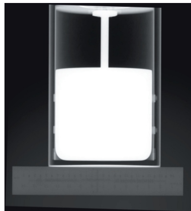
Figure 5. The X-ray picture of the ORTEC GEM100P4-95 HPGGe detector
